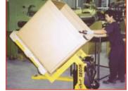
The portable tote box tilter is designed to make the lifting, handling and positioning of small parts containers easy on the worker's back.
